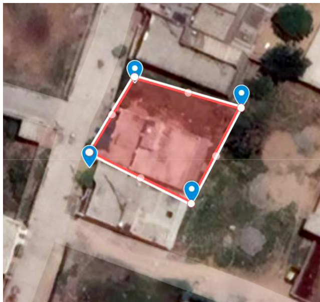
Figure 7 Using Google satellite imagery to rectify a construction source's misplaced polygon mapped by field staff while recording the source
